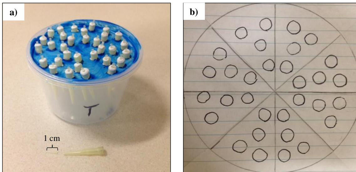
**Figure 7.** Artificial flower construction showing **a)** an assembled flower with all nectaries in place and **b)** sketch of the well template, showing spatial arrangement of the 32 nectaries on the container lid.
