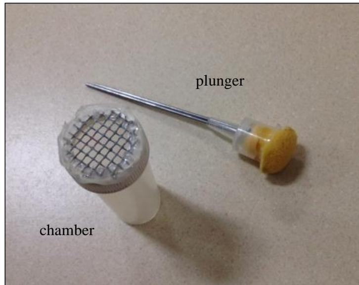
**Figure 9.** Bee squeezer parts used to immobilize bees for marking—modified from a design described in Kearns and Thomson (2001).
